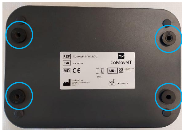
Figure 13. Blind nuts positioned in the four holes of the Electronics Control Unit.
