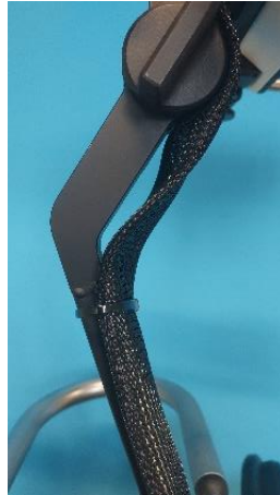
Figure 11. Use of tie wraps.
