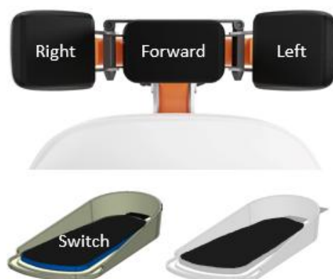
Figure 16. Drive with back head - Switch with one foot.
