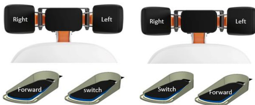
Figure 15. Drive with foot - Switch with foot configuration.
