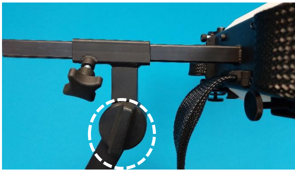
Figure 3. Rotary knob to adjust the inclination of the head array.
