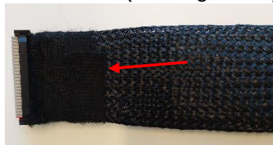
Figure 48. Apply cloth tape.
