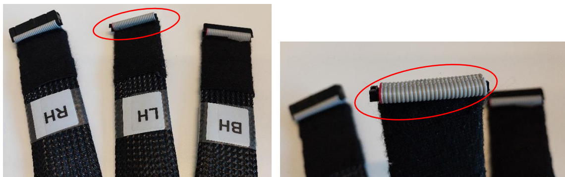
Figure 34. An example of a broken IDC connector.
