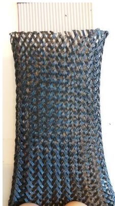
Figure 37. Cut braided sleeve by 4-5 cm.
