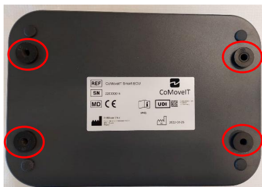
Figure 4. Blind nuts positioned in the four holes of the Electronics Control Unit.
