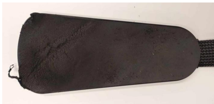
Figure 6. Footpad with damaged cover sticker.
