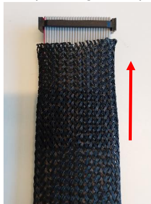
Figure 47. Slide the braided sleeve.
