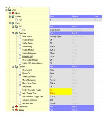
A direction change will occur if the back head pad of CoMoveIT Smart is operated and released. Further operation of the back head pad will result in driving in the newly selected direction. **Fwd / Rev Auto Toggle** must be set to **On**.
