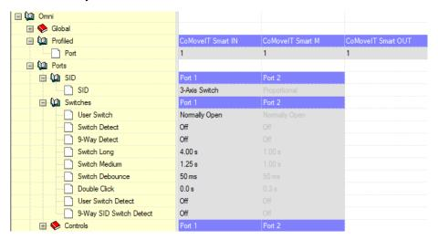
In this configuration, you use CoMoveIT Smart Rnet settings for four-sensor configuration. However, instead of connecting a User Switch Sensor to CoMoveIT Smart, the User Switch (buddy button or similar) is connected to U1 of Omni.
